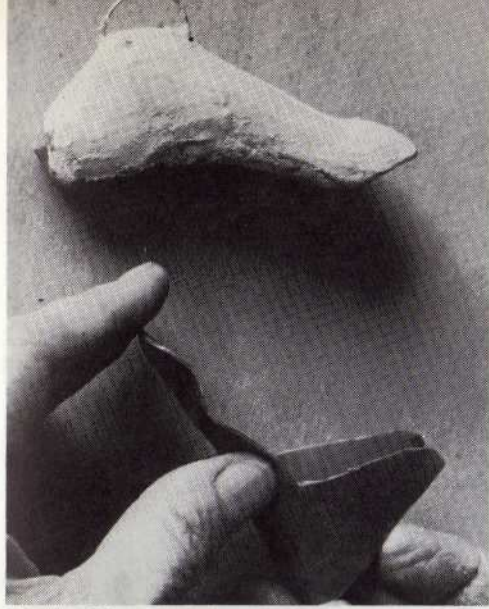
Fig. 91. Sheet lead foot pattern and finished foot with wire joint
