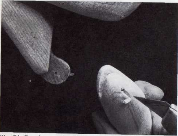
Fig. 74. Carving notch at hole in lower arm
