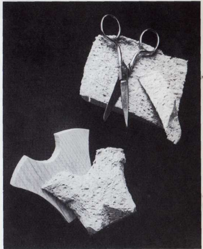
Fig. 99. Cellulose sponge can replace balsa wood as front block
