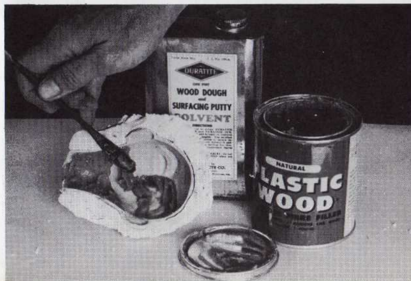
Figs. 43 & 44. Lining the two halves of the mold with plastic wood
