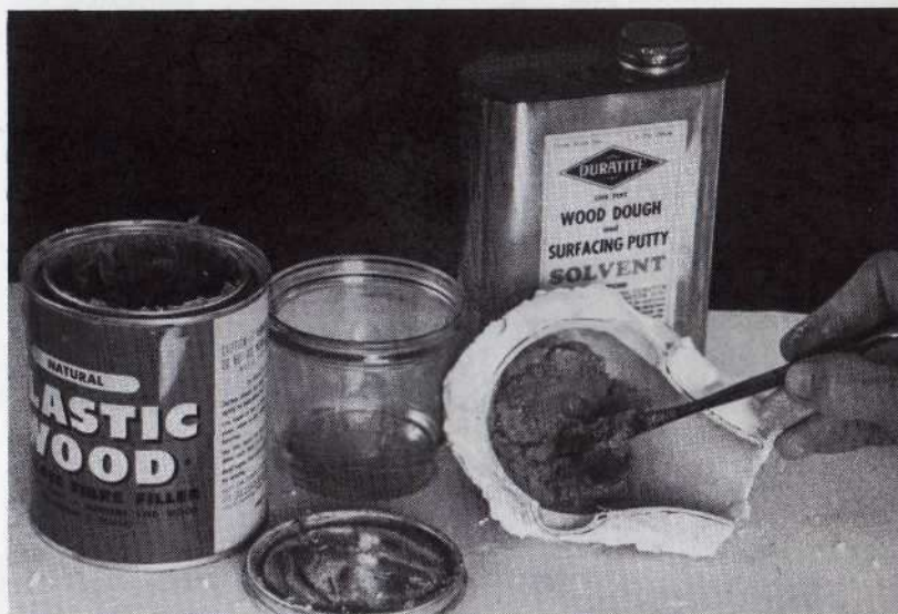
Figs. 43 & 44. Lining the two halves of the mold with plastic wood
