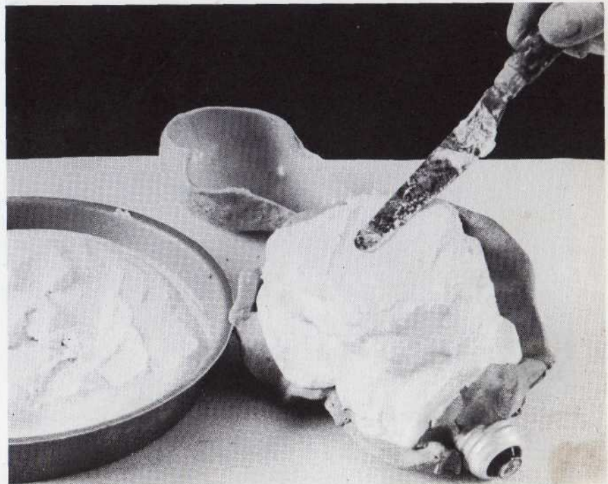
Fig. 39. Spreading plaster on outside of mold
