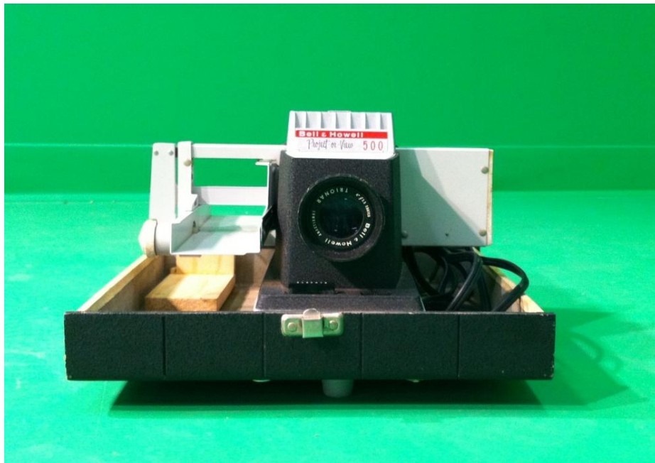
Figure 29 An old Bell & Howell Project 'N' View 500 projector for the shadow projection of the puppet
