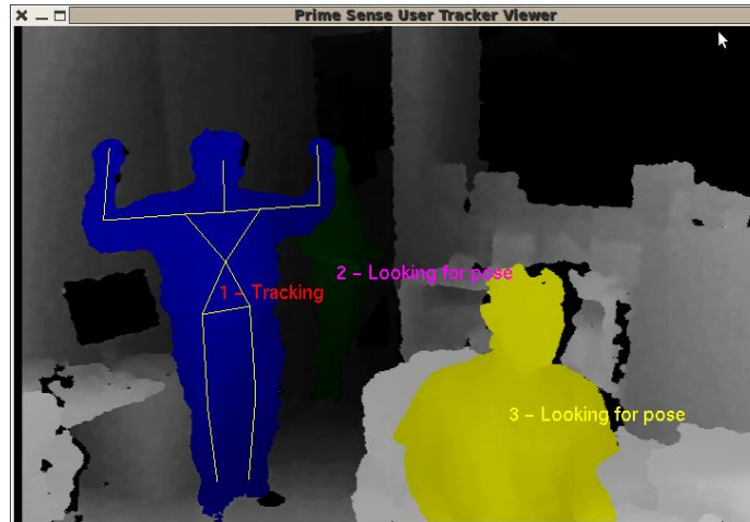
Figure 4 OpenNI allows for tracking users and understanding limb positions
